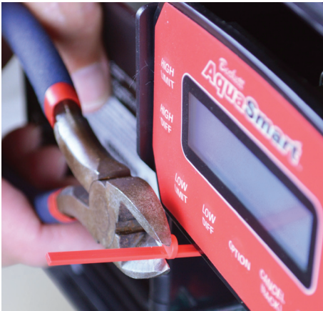
Figure 9 – Clipping the Pushrod to Length
